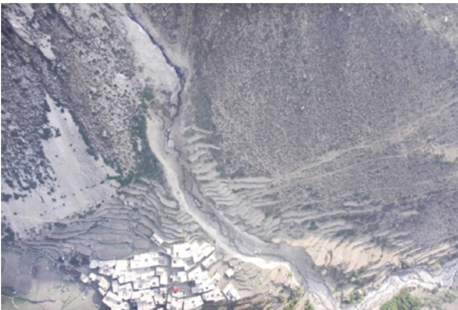
Figure 16: An aerial view captured by an Uncrewed Aerial Vehicle (UAV) shows a deeply incised drainage channel cutting through the rocky steep terrain in the upper section, with pronounced vertical and lateral erosion on the talus fan deposits in the middle and lower sections. Til village is visible in the lower left corner of the image.
